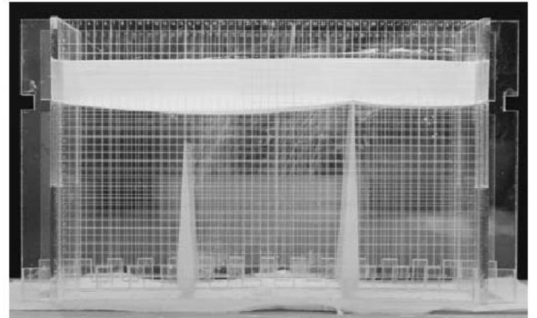
Figure 3: Laser cut rigid mold with elastic base
